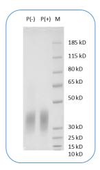
Human PD-1 Protein (C-His-Avi) on SDS-PAGE under reducing condition (P+) and non-reducing condition (P-). The gel was stained for 1 hour with BlinkBlue (catalog 700102). The purity of this protein appears to be greater than 95%.
