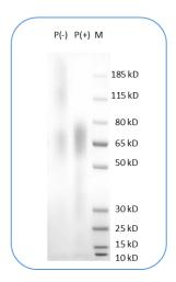
Human CD30 protein (C-His) on SDS-PAGE under reducing condition (P+) and non-reducing condition (P-). The gel was stained for 1 hour with BlinkBlue (catalog 700102). The purity of this protein appears to be greater than 80% based on reducing conditions.
