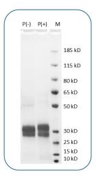
Human 4-1BB Protein (C-His-Avi) on SDS-PAGE under reducing condition (P+) and non-reducing condition (P-). The gel was stained for 1 hour with BlinkBlue (catalog 700102). The purity of this protein appears to be greater than 95%.
