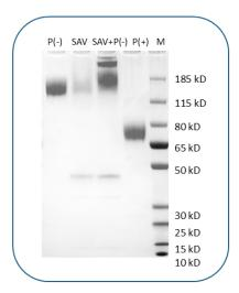
Human B7-1 (CD80) Protein (C-His-Avi) was biotinylated in vitro using BirA ligase. SDS-PAGE analysis under reducing (P+) and non-reducing (P-) conditions shows the protein has a purity greater than 95%. A gel shift assay using co-incubation with streptavidin indicates that the biotinylation efficiency of Human B7-1 protein exceeds 90%.
