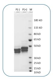
Mouse OX40 (C-His) on SDS-PAGE under reducing condition (P+) and non-reducing condition (P-). The gel was stained for 1 hour with BlinkBlue (catalog 700102). The purity of this protein appears to be greater than 95% based on reducing conditions.
