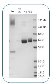
Biotinylated HexA/B heterodimer (HexA-His/HexB-FLAG) final product on SDS-PAGE under non-reducing (P-) and reducing (P+) conditions. The purity of HexA/B heterodimer (HexA-His/HexB-FLAG) is greater than 95%. Based on Gel shift Assay by co-incubation with Streptavidin, biotinylation efficiency is >95% for HexA/B heterodimer
